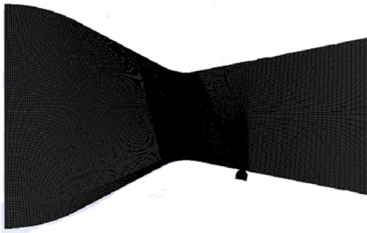
Fig. 2 Grid system in the computational domain of a CD nozzle
