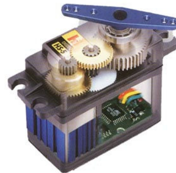
Fig. 4 Constructive aspect of a servomotor
