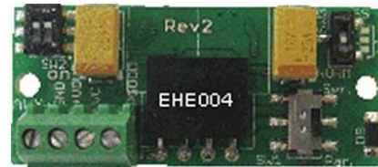
Fig. 6 Buck boost circuitry as power electronics circuit
