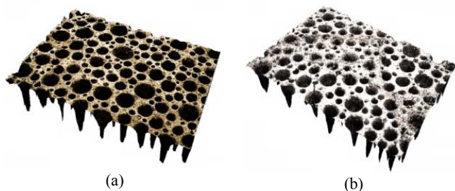
Fig. 5 3D confocal laser micrographs before (a) and after (b) the six immersions
