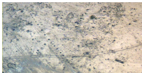
Fig. 26 Micrograph of 25% groundnut shell filler
