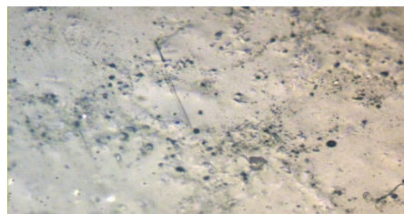
Fig. 20 Micrograph of 15% groundnut shell filler
