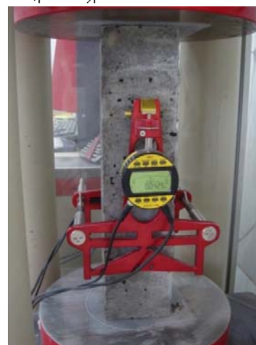
Fig. 3 Schema and practical measurement of modulus of elasticity [15]
