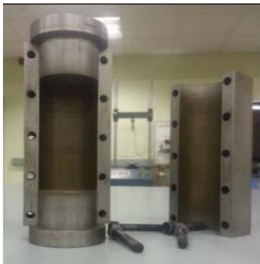
Fig. 6 Constant Volume Mould Used to Prepare the Soil Specimens for UCS Tests
