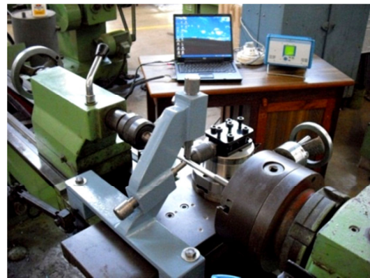
Fig. 2 Experimental set-up of turn assisted deep cold rolling process
