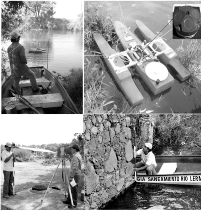
Fig. 4 Getting hydrometrical and topographical information by a Doppler effect acoustic profiler (shown at the top) and a total station
