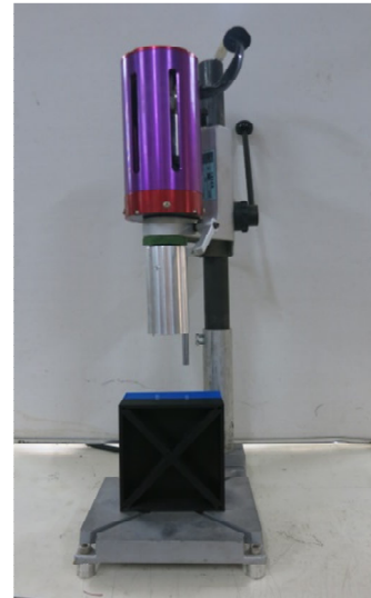
Fig. 8 Ultrasonic tube flanging specialized station
