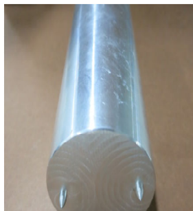
Fig. 6 The real horn made by aluminum
