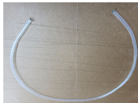
Fig. 10 The flanged tube of Teflon with 4mm diameter
