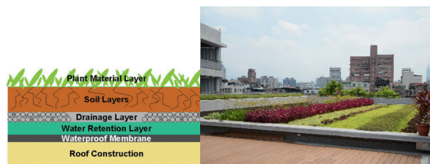
Fig. 2 The green roof configuration and environment images
