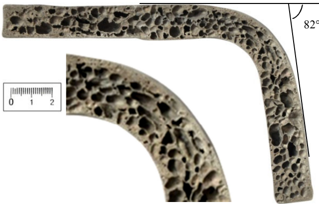
Fig. 4 The specimen, on which free bending was performed in 656°C
