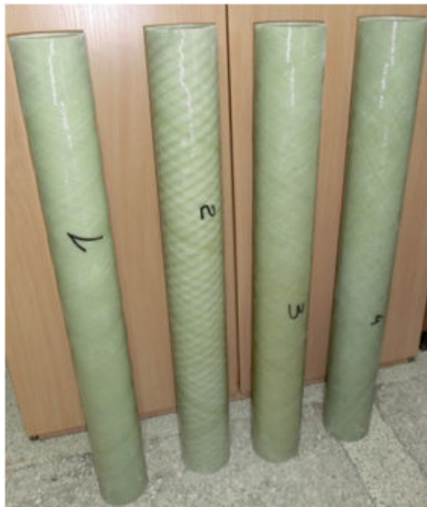
Fig. 2 Prepared composite samples before testing
