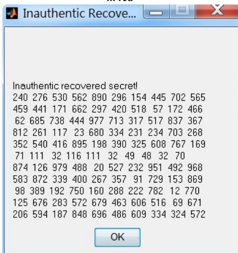
Fig. 8 A dialog shows the value inconsistency of computed 11 sets of coefficients extracted for the attacked stego-file
