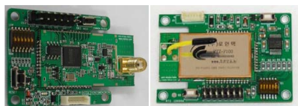
Fig. 1 Wireless modules with JN5139 microcontroller
