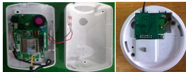
Fig. 5 CO and smoke detector with wireless module
