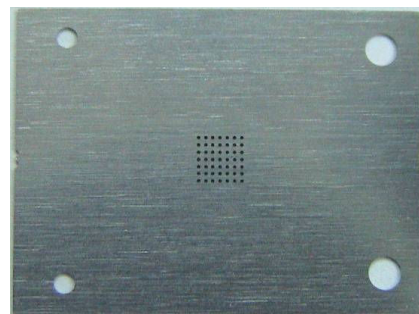
Fig. 15 The fabricated stainless steel channel plate II
