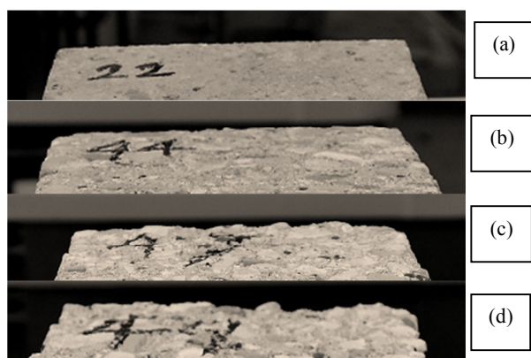
Fig. 2 Cube sample 22 before immersion (a), cube samples 44 after 28 days (b), cube sample 47 after 42 days (c) and cube sample 49 after 56 days of immersion (d)
