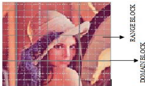
Fig. 2 (b) Lena image partitioned into range and domain blocks
