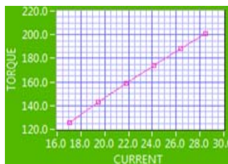
Fig. 5 Torque vs current characteristics of induction motor
