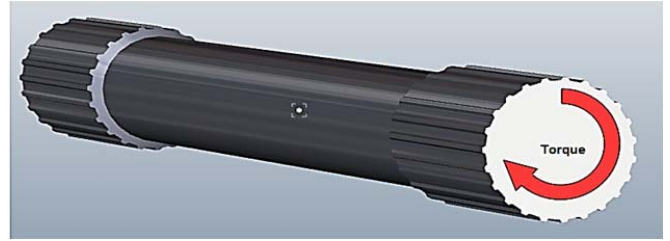
Fig. 2 Forces acting on axle of JD955 and JD1055 in static displacements
