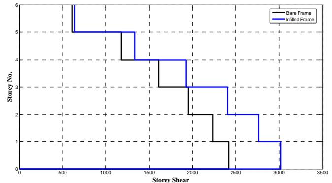
Fig. 4 Storey shear forces dynamic RS X-dir
