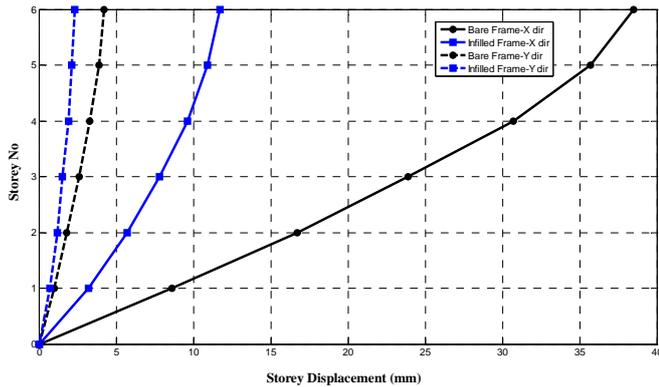
Fig. 5 Storey displacements in X and Y direction throughout the height of building for two building models under RS loading in X-dir
