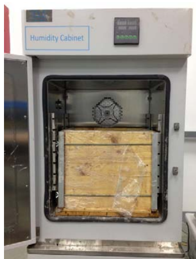
Fig. 2 Insulated Plywood Box inside an Environmental Chamber
