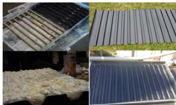
Fig. 1 Flat plate collector (FPC)
