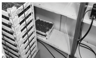
Fig. 2 Column of crates placed on the vibrating table and contained in cooling cell
