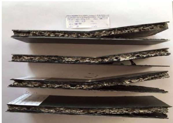
Fig. 12 Collapsed sandwiches named SWAF after the bending tests at different support span values (top to bottom: L = 55, 70, 80 and 125 mm)
