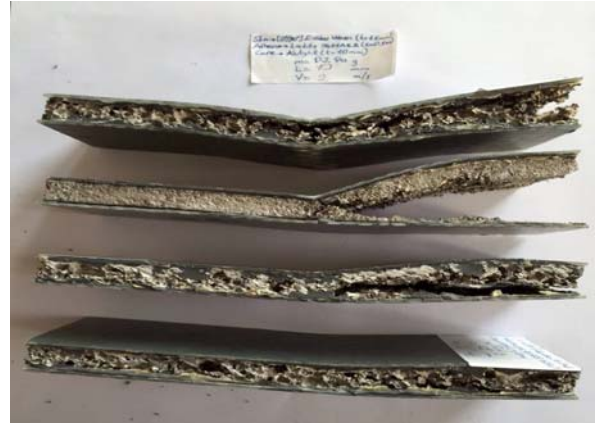
Fig. 11 Collapsed sandwiches named EWAT after the bending tests at different support span values (top to bottom: L = 55, 70, 80 and 125 mm)
