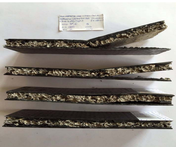
Fig. 10 Collapsed sandwiches named EWAFF after the bending tests at different support span values (top to bottom: L = 55, 70, 80 and 125 mm)
