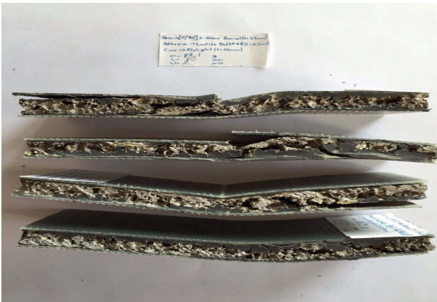
Fig. 9 Collapsed sandwiches named EBSAT after the bending tests at different support span values (top to bottom: L = 55, 70, 80 and 125 mm)
