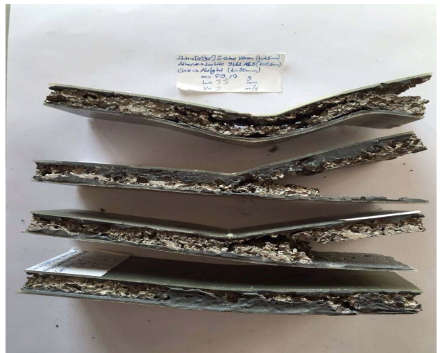
Fig. 13 Collapsed sandwiches named SWAT after the bending tests at different support span values (top to bottom: L = 55, 70, 80 and 125 mm)
