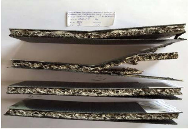
Fig. 8 Collapsed sandwiches named EBSAF after the bending tests at different support span values (top to bottom: L = 55, 70, 80 and 125 mm)
