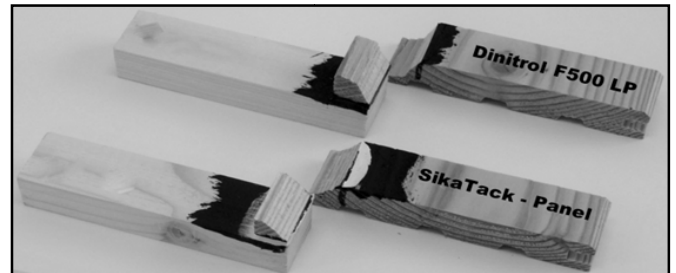
Fig. 10 Determination of the tensile lap – shear of bonded assemblies – Specimen failure during testing
