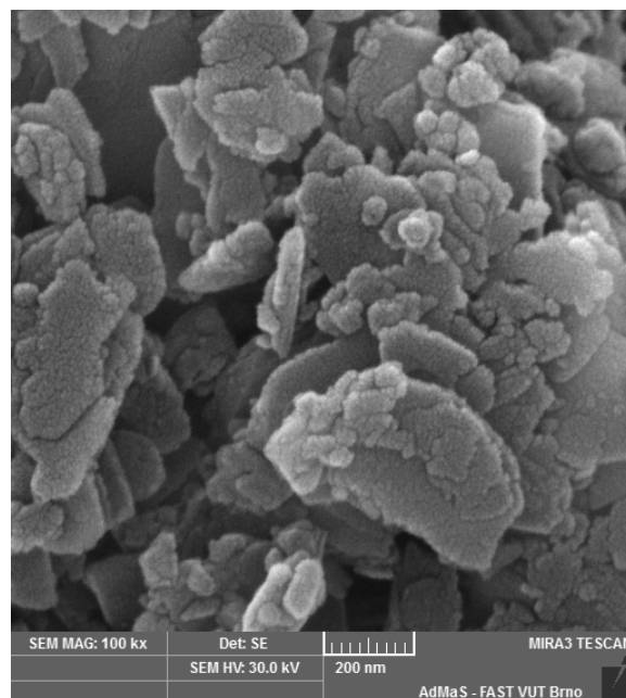
Fig. 2 A view of the structure of the zeolite
