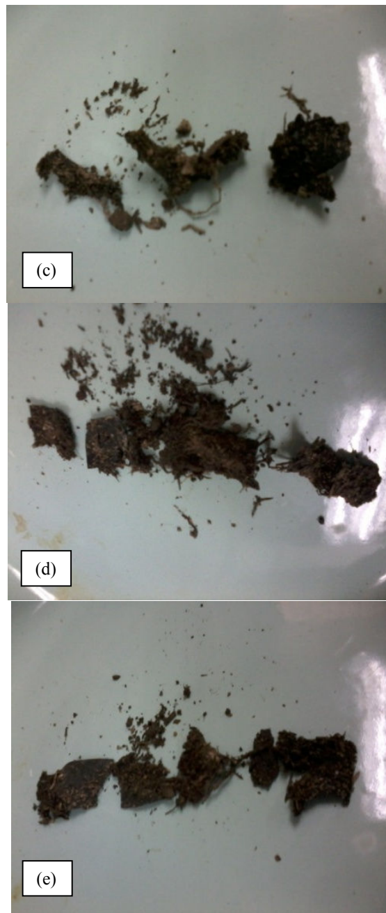
Fig. 3 Image of degraded hybrid films after 60 days of soil exposure (a) polybag 20%, (b) polybag 30%, (c) polybag 40%, (d) polybag 50%, (e) polybag 60%,
