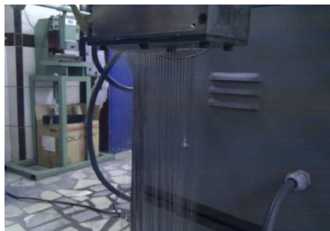
Fig. 2 Coat- Hanger die mounted on extruder and produced fibers
