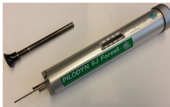
Fig. 1 Pilodyn 6J indentation device
