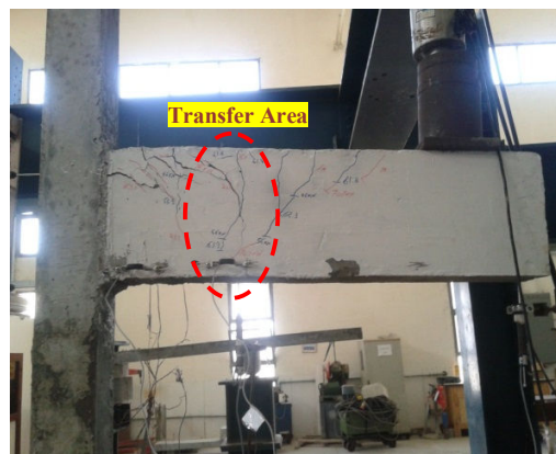
Fig. 15 Cracks at the failure of SP4
