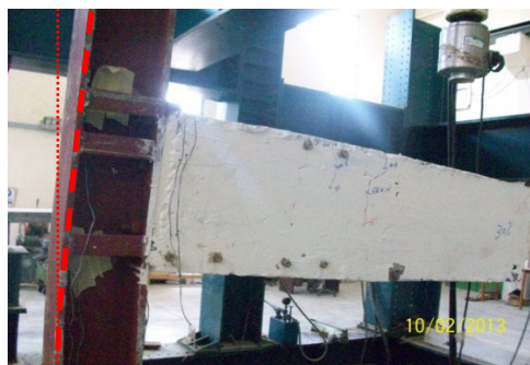
Fig. 13 SP2; Beam flexural cracks and column deformed shape
