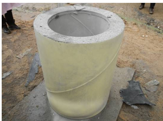
Fig. 8 Litter bin after real blast test
