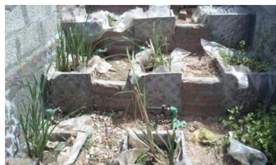
Fig. 2 Mesocosms set up of constructed wetland built in open field environment
