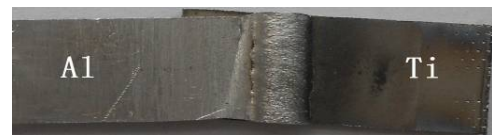
Fig. 8 Fracture location of tensile test
