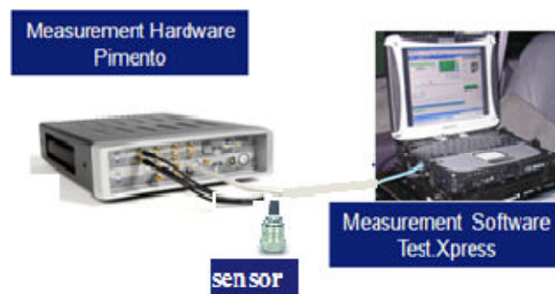
Fig. 4 Typical setup of transducer-data acquisition pair
