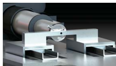
Fig. 5. Load cell mounted onto the actuator
