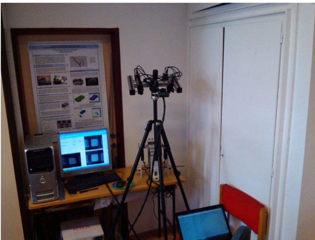
Fig. 7 Combination of VIALUX system & bi-axial stress measuring
