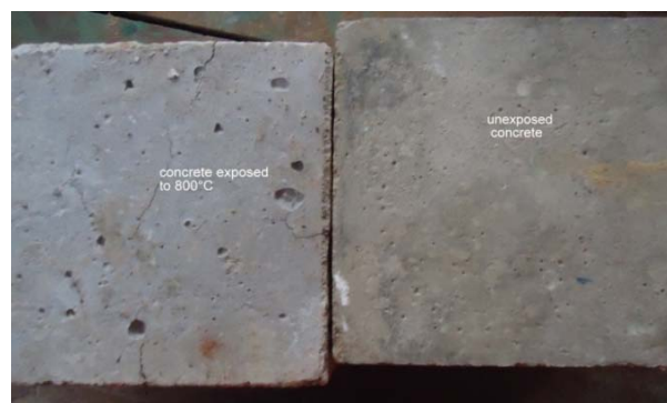
Fig. 2 Concrete exposed to 800°C
