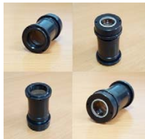
Fig. 2 Optical system of star tracker experimental model
