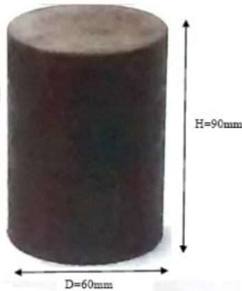
Fig. 2 Sample prepared; D= 60 & H= 90 mm
