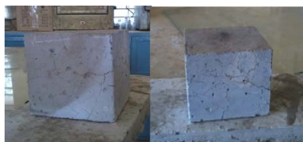
Fig. 3 Concrete specimens subjected to 800°C
