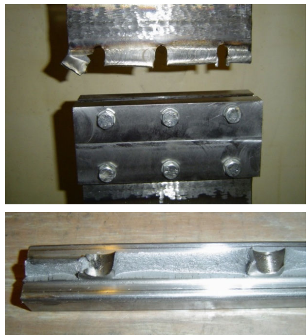
Fig. 5 Typical failure mechanism: plate fracture in place of bolt holes
