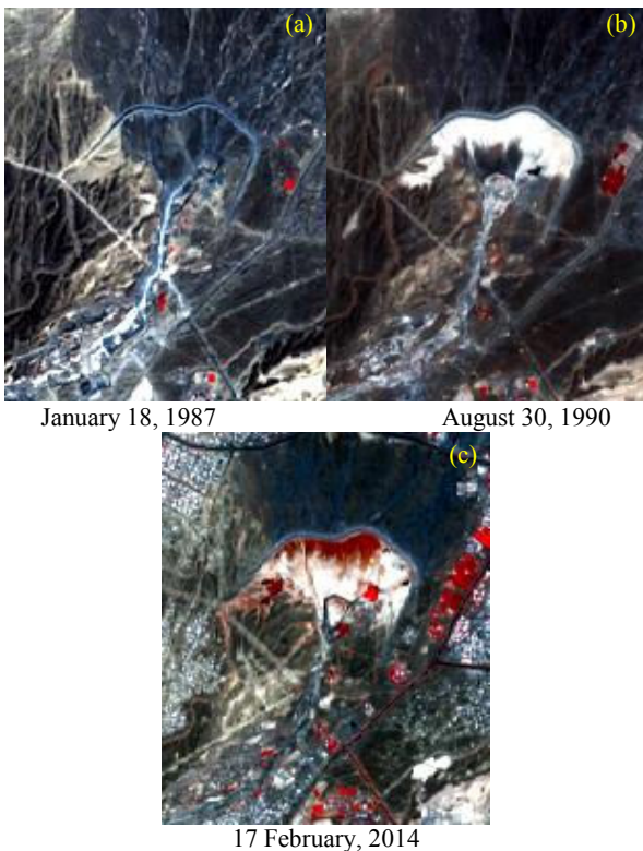
Fig. 5 (a) (c) Landsat data shows the siltation (white) and vegetation (red) in the Alkhod dam
