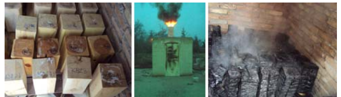
Fig. 2 The image where placements of wooden samples, the moment of fire and after fire exist
