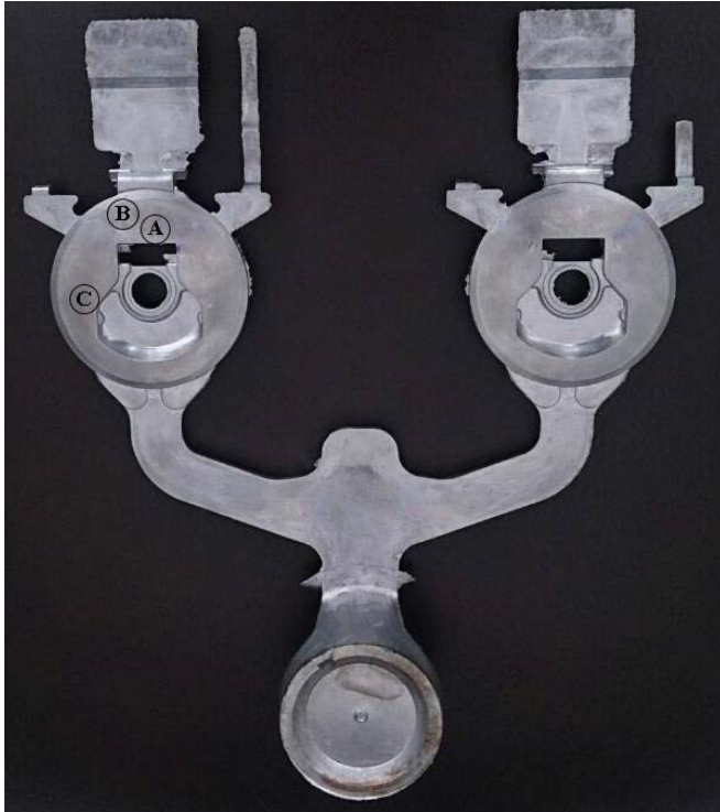
Fig. 1 A HPDC part for motorcycle fuel caps
