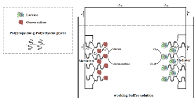
Fig. 2 Scheme of the bioelectrochemical reactions for the proposed enzymatic fuel cell
