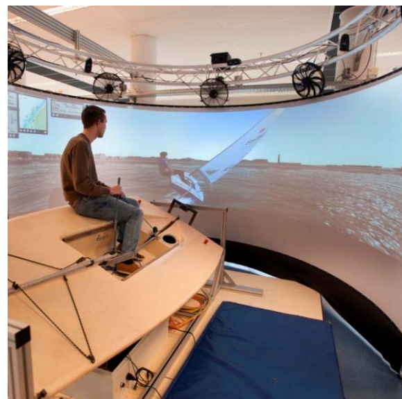
Fig. 9 InnoSportLab’s Yacht Simulator
