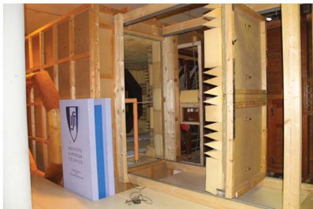
Fig. 9 IST's anechoic room
