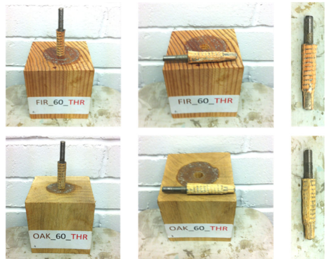
Fig. 13 Failure mode in Oak (bottom) and Douglas Fir (above) samples with rough and threaded borehole after being tested by a pull-out test
