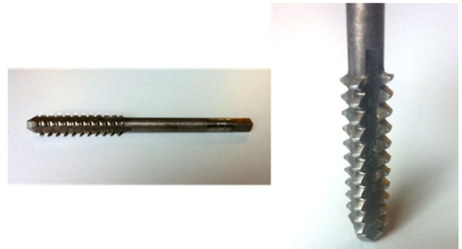
Fig. 3 Specific drill bit for woodworking used to create the new threaded hole shape
